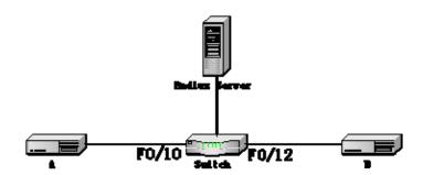
Host A connects interface f0/0 of the router; host B connects interface f0/12 of the switch. The IP address of the radius server is 192.168.20.2 and the radius key is TST. The authentication of interface f0/10 adopts the remote radius authentication and the user binding function. The authentication of interface f0/12 adopts the local authentication without user binding, however, the EAP authentication mode and multi-host authentication will be employed.
